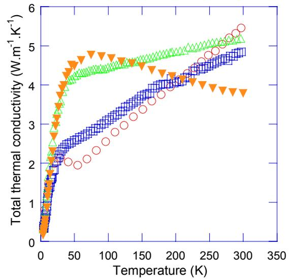
Figure 2: Temperature dependence of the total thermal conductivity for the  $\text{Mo}_3\text{Sb}_7$  ( $\circ$ ),  $\text{Mo}_{2.78}\text{Ru}_{0.22}\text{Sb}_7$  ( $\square$ ),  $\text{Mo}_{2.5}\text{Ru}_{0.5}\text{Sb}_7$  ( $\triangle$ ) and  $\text{Mo}_{2.2}\text{Ru}_{0.8}\text{Sb}_7$  ( $\nabla$ ) compounds.
