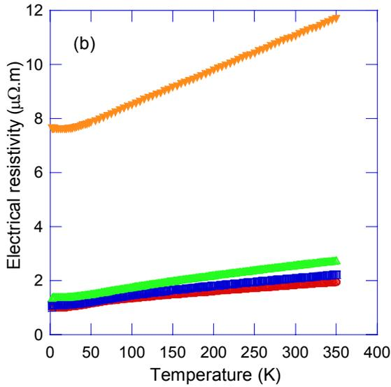
Figure 1: Temperature dependence of the thermopower (a) and electrical resistivity (b) for the  $\text{Mo}_3\text{Sb}_7$  ( $\circ$ ),  $\text{Mo}_{2.78}\text{Ru}_{0.22}\text{Sb}_7$  ( $\square$ ),  $\text{Mo}_{2.5}\text{Ru}_{0.5}\text{Sb}_7$  ( $\triangle$ ) and  $\text{Mo}_{2.2}\text{Ru}_{0.8}\text{Sb}_7$  ( $\nabla$ ) compounds.
