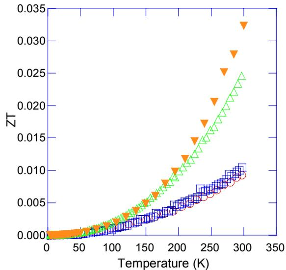
Figure 2: Temperature dependence of the dimensionless figure of merit  $ZT$  for the  $\text{Mo}_3\text{Sb}_7$  (○),  $\text{Mo}_{2.78}\text{Ru}_{0.22}\text{Sb}_7$  (□),  $\text{Mo}_{2.5}\text{Ru}_{0.5}\text{Sb}_7$  (△) and  $\text{Mo}_{2.2}\text{Ru}_{0.8}\text{Sb}_7$  (▽) compounds.
