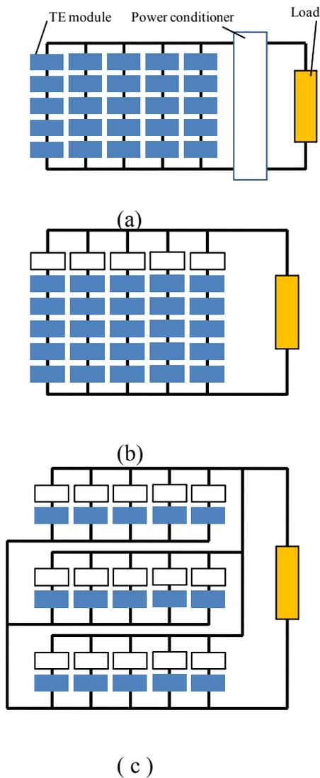
Fig.1 Variation of TEG systems with MPPT power conditioner: (a) single converter system (b) String converter system (c) module converter system.
