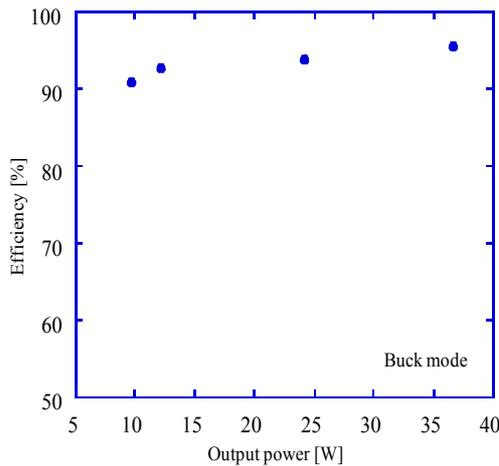
Fig.3 Output power vs conversion efficiency
