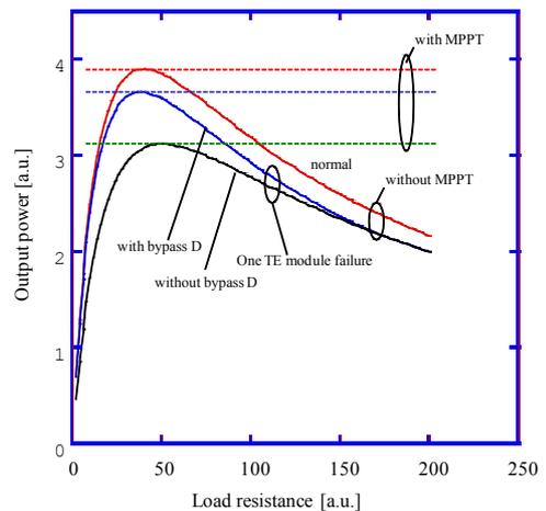
Fig.5 Effect of bypass diode on output power vs load resistance.
