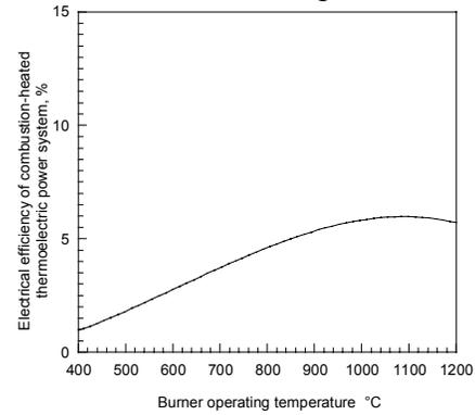
Figure 4. System electrical efficiency vs burner (heat source) operating temperature
