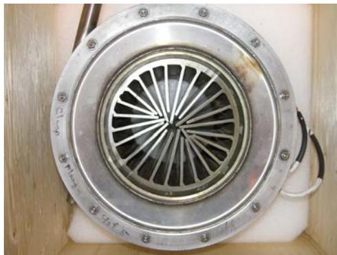
Figure 3. Heat-conducting fins on module's inner wall to enhance heat transfer from gaseous combustion products to thermoelectric module
