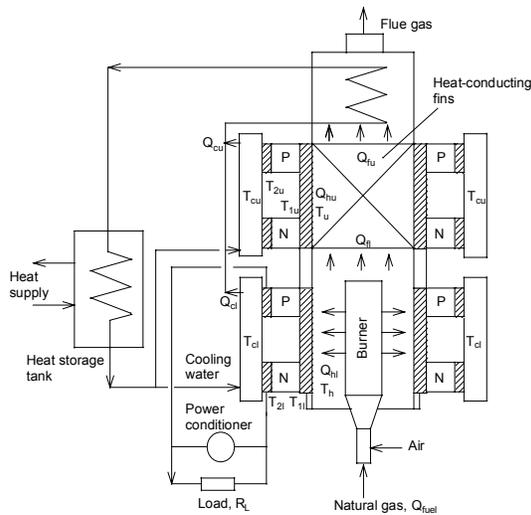
Figure 1. Gas-fired micro-cogeneration system using two thermoelectric modules
