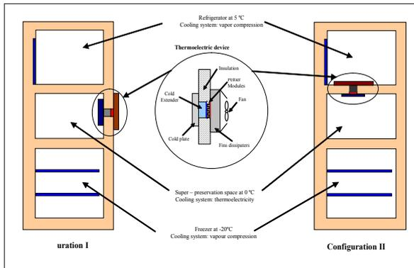
Figure 1. Sketches of the hybrid domestic refrigerator. Configurations I and II.
