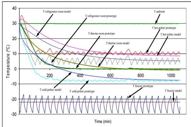
Figure 2. Comparison of the results from the prototype and the computational model.
