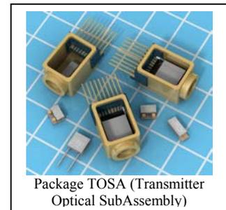
Package TOSA (Transmitter Optical SubAssembly)
