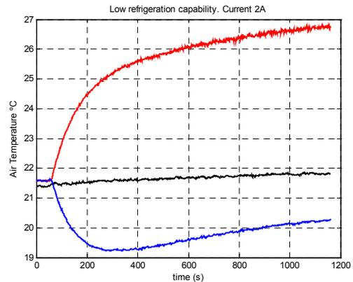
Figure 4: Result of undersized refrigeration
