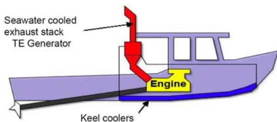
Figure 2. Exhaust heat recovery thermoelectric generator on a boat.
