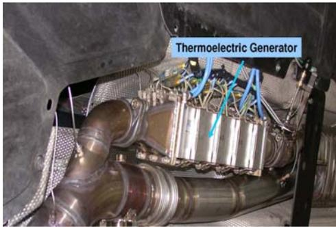
Figure 7. Installation of TEG in the BMW
