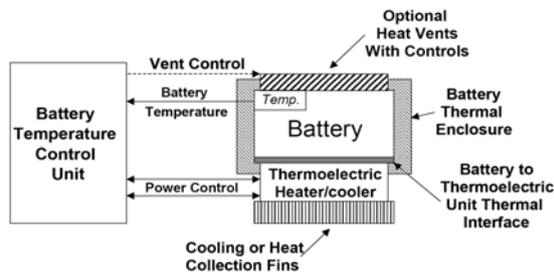
Figure 8. Schematic of a battery temperature control system.
